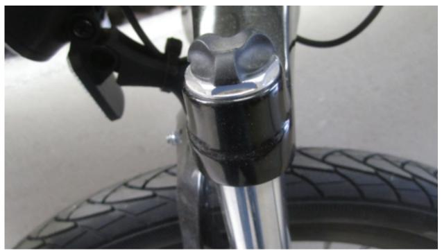
• Lock Out Control - Lockout the fork so there is no suspension travel by turning the knob on the top of the right fork leg. Turn counterclockwise to lock out the fork.
