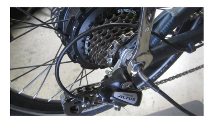
**4.** Locate the motor disconnect weather proof plug on the right side of the bike frame, 6 inches foreward of the rear axel. Pull the plug apart and do not twist. When reconnecting push but do not twist. Cut the wire tie holding the cable in the cable mounting tab.
