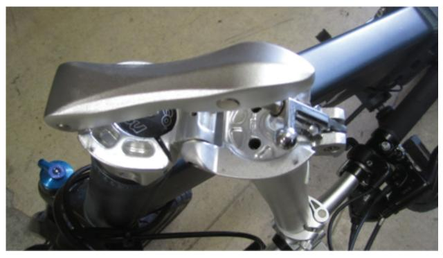
**3.** Fold the frame at the middle by lifting the silver bar.
