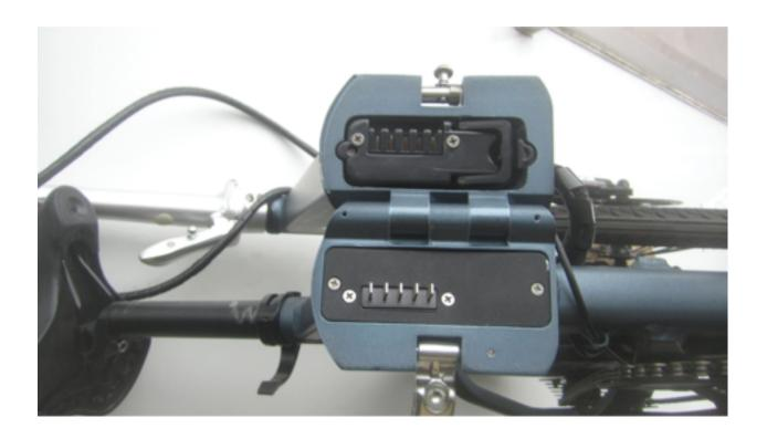
**2.** Insert the key into the key lock, turn the key to unlock the battery, and pull the battery out usaing the handle.
