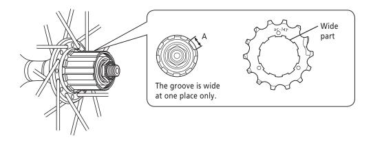
• For installation of the HG sprockets, use the special tool TL-LR15 / LR10 to tighten the lock ring.
