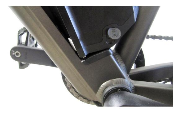
**2.** Then move the battery sideways into the lock position. The S/T's battery mounts on the downtube of the bicycle from the left side.
