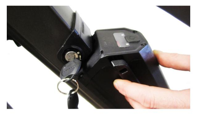
**3.**The battery will be a tight fit. ALWAYS confirm the battery is locked in place by pulling the top of the battery sideways. By pulling on the battery, this will assure the battery has locked into position.
