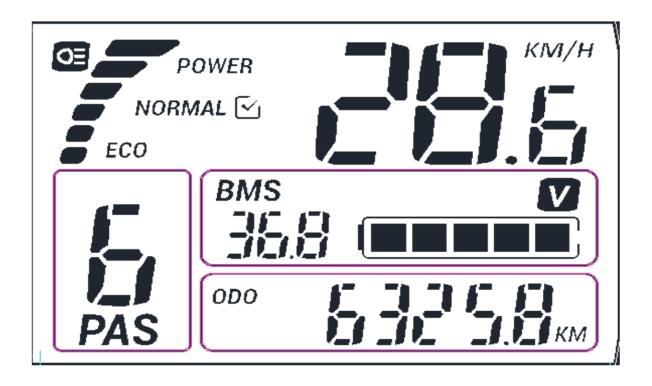
**Current Display** - Shows discharge current, each mark is 2amps
