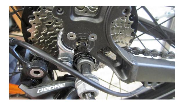
**3.** Now check to make sure the chain is not in the way and align the wheel above (below if bike is on kick stand and not upside down) the dropouts and pay attention to the lining up of the disk brake rotor into the brake caliper (between the pads).
