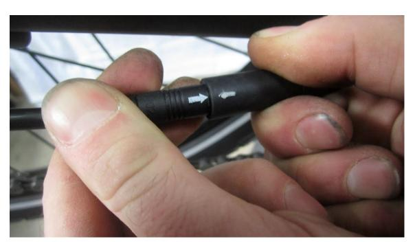
**6.** On each axle nut there is a rubber nut protector, remove these protectors simply by pulling on them. On the wired side of the axle, slide the rubber protector up the wire only a few inches.
