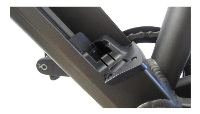
**1.**To mount the battery, you would first slide the base of the battery into the frame's lower docking mount (closest to the crankset)
